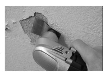
**NOTE:** The scraping blade is designed for scraping soft materials from flat surfaces. Ensure you get the correct angle and only apply light pressure to avoid cutting the surface.
