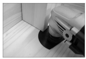
NOTE: If using the saw attachments for plunge cuts, only use the saw on soft materials such as softwood and plaster boards. Always check that there are no nails or screws in the workpiece before cutting.
